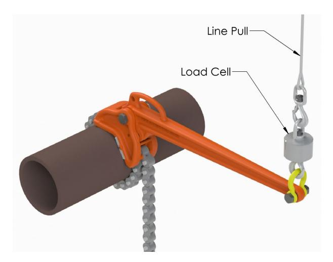
WARNING: The pipe must be constrained to prevent excessive deflection of the pipe. Excessive deflection of the pipe could lead to side loading. Side loading will result in premature failure of the tong and/or chain which may result in injury or death.
