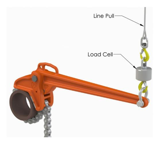
WARNING: The pipe must be constrained to prevent excessive deflection of the pipe. Excessive deflection of the pipe could lead to side loading. Side loading will result in premature failure of the tong and/or chain which may result in injury or death.
