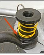
When using offset striking wrenches, place the notch of the retaining plate facing the wrench handle as shown.
