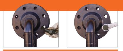
Find a bolt hole aligned enough for the tapered shaft to fit thru and turn.
