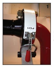
1. Wrap the strap around the bolted flanges prior to unbolting. Feed the free end over the top of the two adjustment lock pins.
