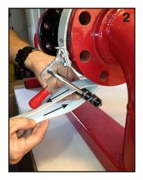
2. Then feed the free end back through the tension adjustment bolt, in between the two adjustment lock pins.
