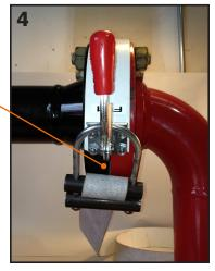
5. Engage the tension clamp. If the tension clamp is difficult to close loosen the strap slightly and try again. The strap is tightened correctly when the edges are firmly seated around the flanges and does not slip when pressure is applied at any point.
