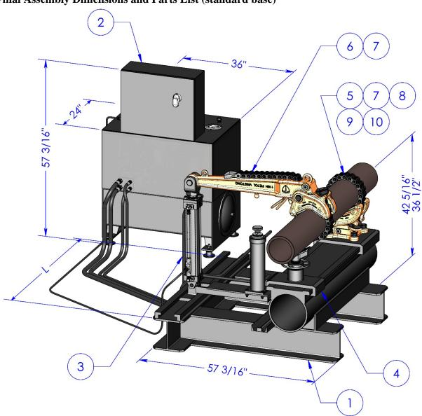
Final Assembly Dimensions and Parts List (skid mount)
