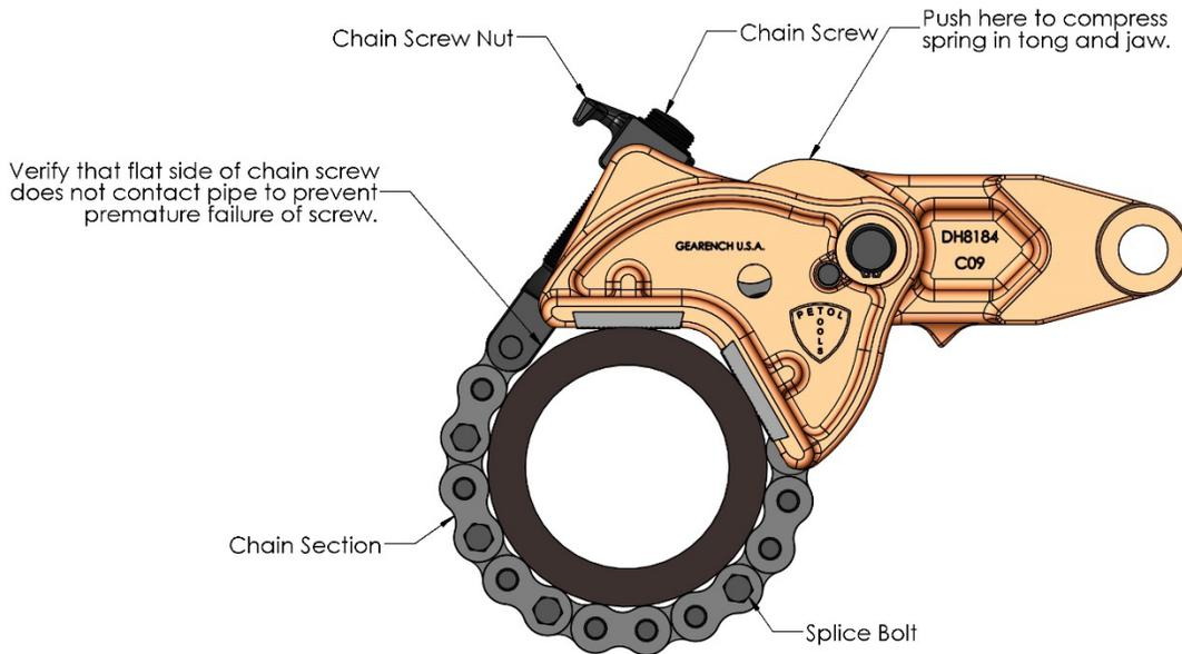
**Warning! The pipe must NOT contact the side of the chain screw as shown above. Contact will cause premature breakage of the chain screw and could cause injury or death. If the chain screw contacts the pipe, the chain MUST be lengthened by adding 2 pitches of chain.**
